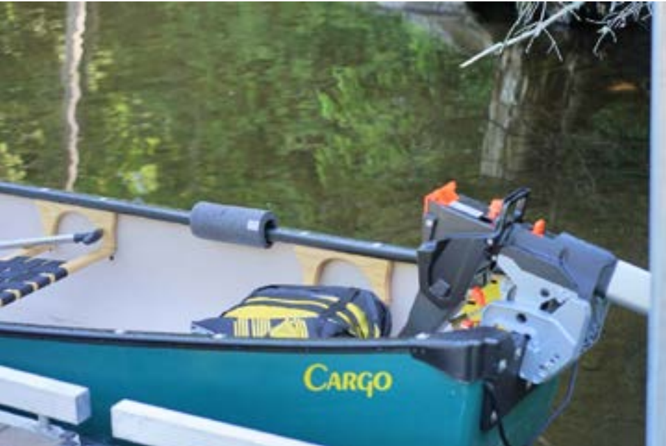
The electric Torqeedo motor attached to the boat without the battery.
