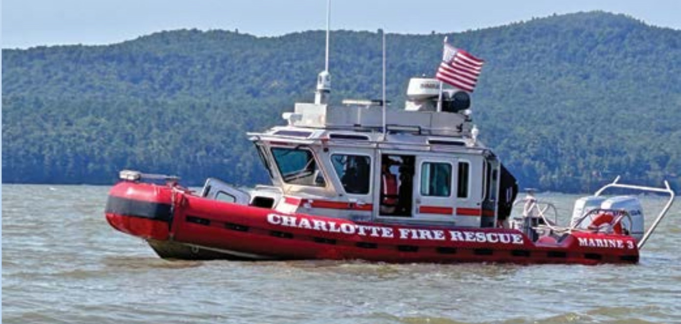
Courtesy photo Charlotte Volunteer Fire and Rescue Service's Marine 3 is a defender class response boat, capable of 45 knots and handling 4-to-6-foot waves.
